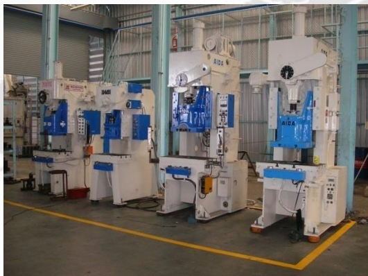
Pressing Machine 32 Units 20-400 tons
